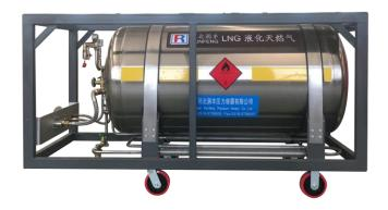
The production of horizontal type cryogenic cylinder a dopt advanced technologies and processes, complianc e to the Quality Assurance System strictly. The cylinde r contains stain steel inner vessel,outer vessel,high vac uum insulation,inner vaporizer and the valves pipes s ystem. It wildly used in **electronics,chemical, weldin g industries.**
